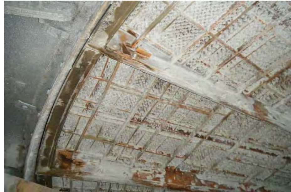
Cold-end baskets with 15 years operation + 1 year of Br addition
